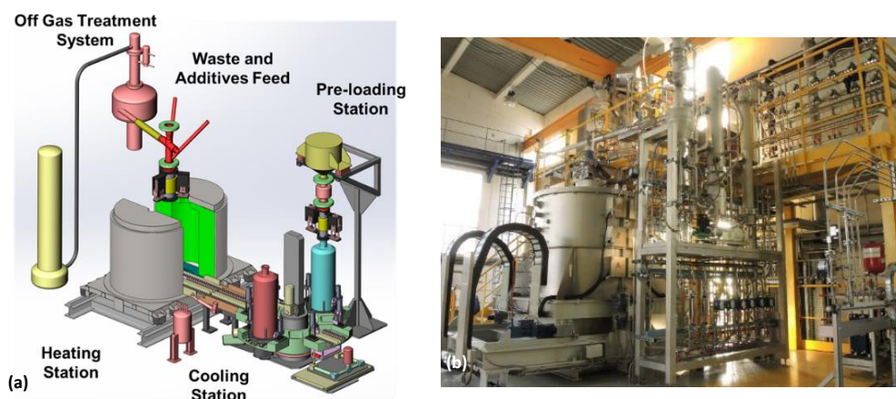
Figure 4. (a) Schematic diagram of the DEM & MELT process. (a) DEM&MELT scale 1 pilot unit built and commissioned at CEA Marcoule
