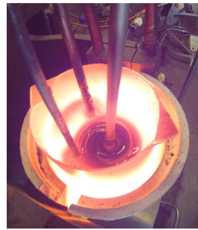
Vitrification of simulated nuclear waste at experimental scale, with a mechanical agitator
