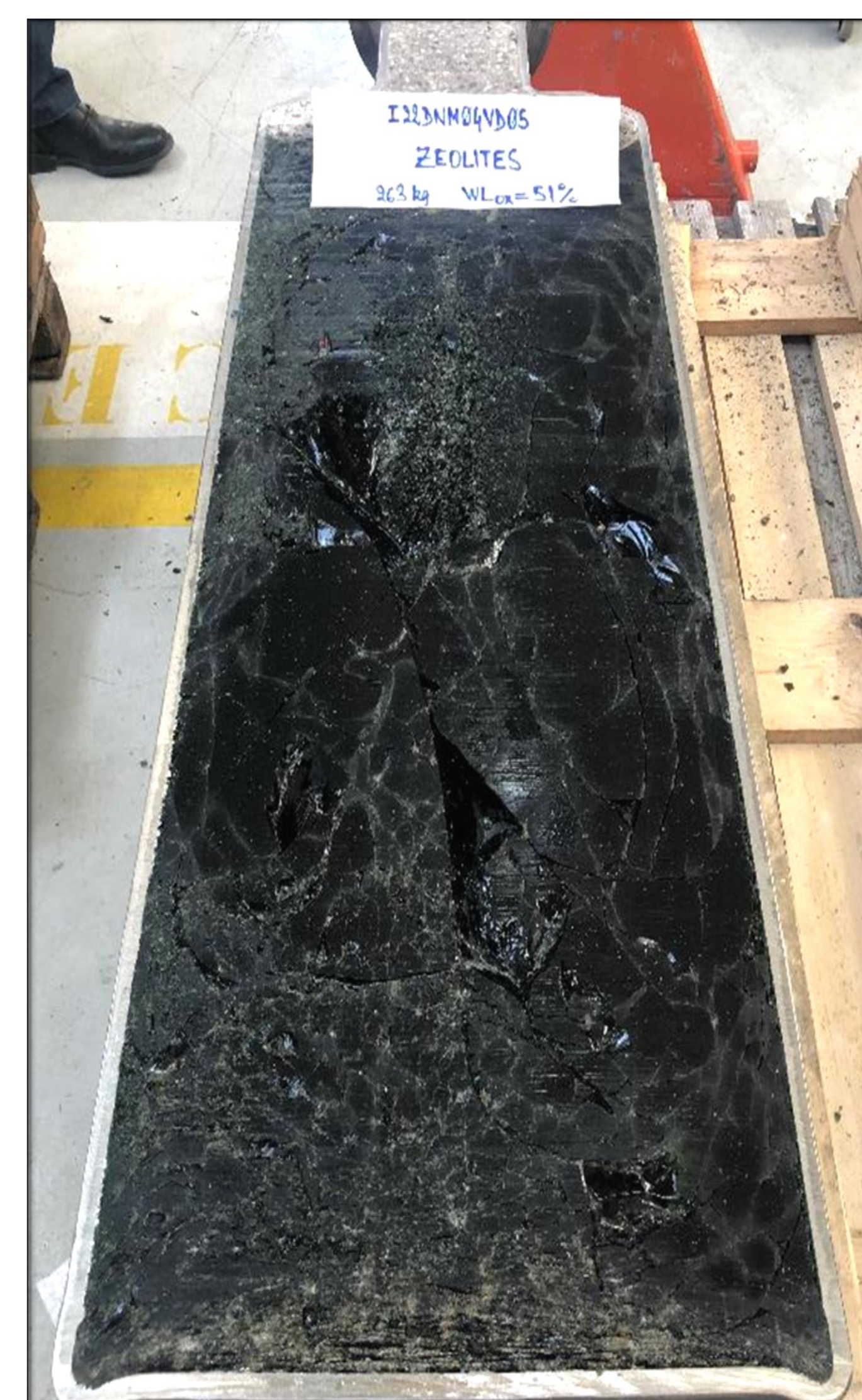
Half-cut CAN 263 kg of final glass WL = 59,1% of zeolite
