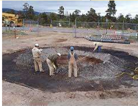
Measuring the monolith created by the planar melt cold test at Los Alamos National Laboratory.
