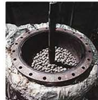
Ball-type thermal decomposer (source: HP of NGK)
