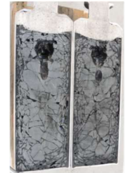
Waste form obtained from test with Dem&Melt (51 wt% WL)
