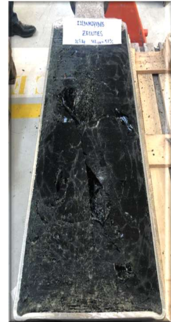
Half-cut CAN 263 kg of final glass WL = 59,1% of zeolite
