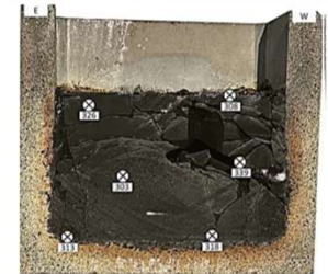
Melter inside during heating and vitrified product
