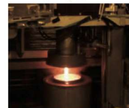
Fig. 4 Appearance of a cold crucible induction melter (CCIM)
