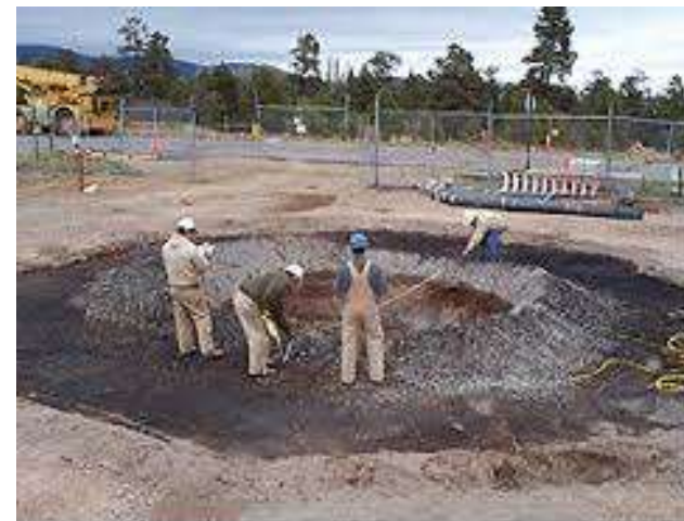
Measuring the monolith created by the planar melt cold test at Los Alamos National Laboratory.
