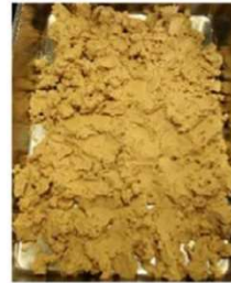
Thermal decomposition of simulated spent resin
