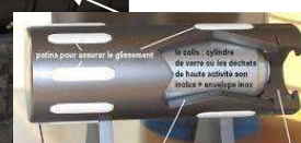
Low carbon steel disposal overpack (~ 63 mm thickness and ceramic skates) to avoid radionuclide release during thermal phase (several hundred years)
