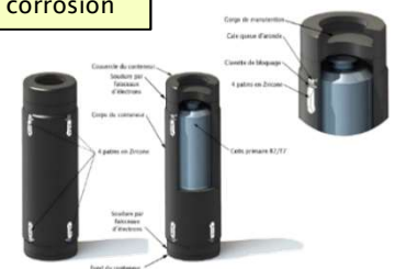
Low carbon steel disposal overpack (~ 63 mm thickness and ceramic skates) to avoid radionuclide release during thermal phase (several hundred years)
