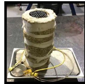
SCMS heat exchanger engineering scale test
