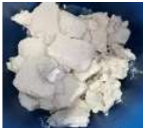
Waste surrogate made by coprecipitation and filtration, same as the real ALPS slurry
