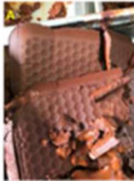
Waste surrogate made by coprecipitation and filtration, same as the real ALPS slurry
